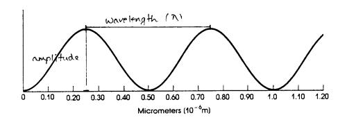
1. Given the distance scale, in micrometers,  $\mu m$  (1.0  $\times$  10<sup>-6</sup>m), shown in the figure, what is the value, in meters per wave, of the wavelength?
